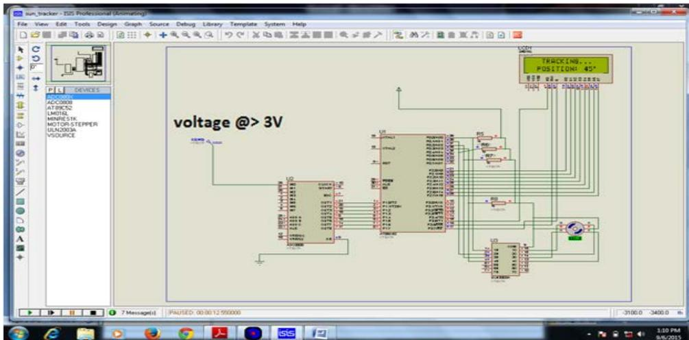
Fig 4.3: LCD showing position of panel at  $V_{IN}$  greater than 3V.
