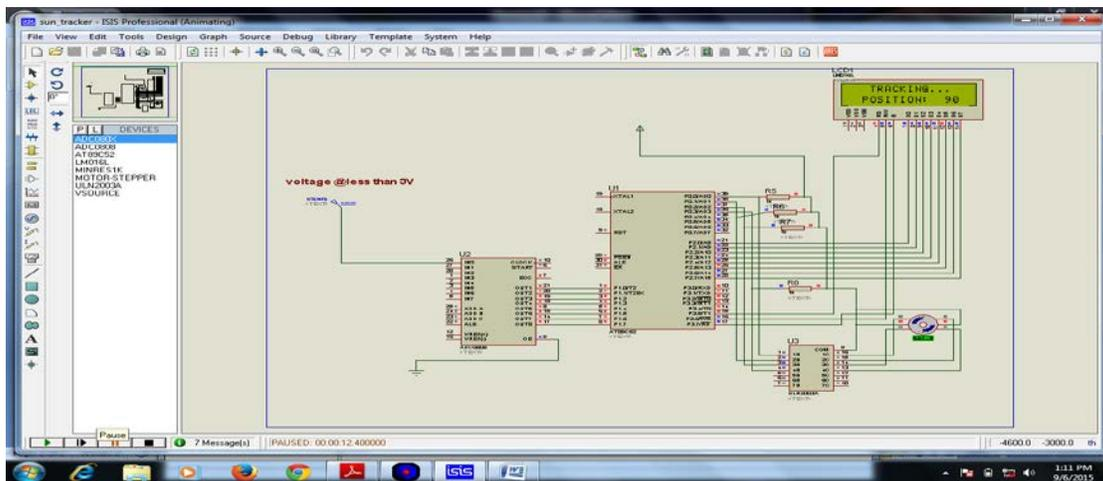
Fig 4.5: LCD showing position of panel at  $V_{IN}$  greater than 3V.
