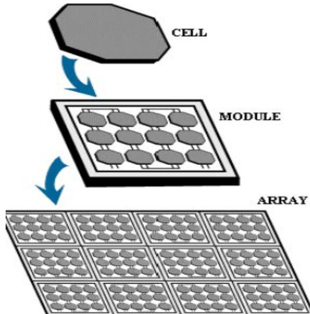
**Fig 2.2:** solar cell basic arrangement
