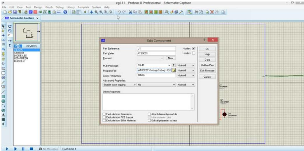
Fig 4.2: load source code into microcontroller
