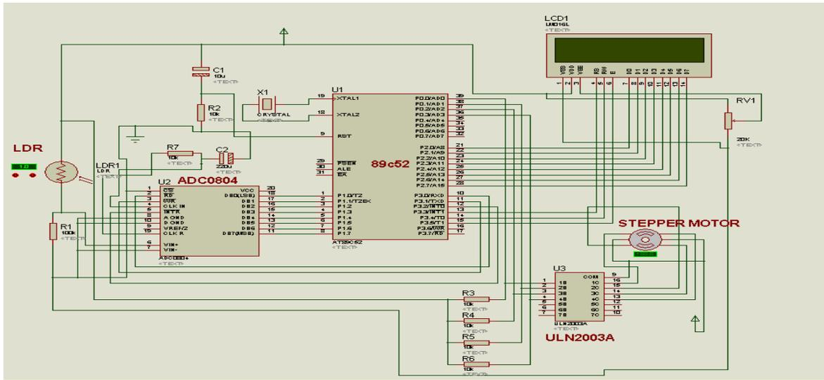
**Fig 4.1:** System circuit diagram
