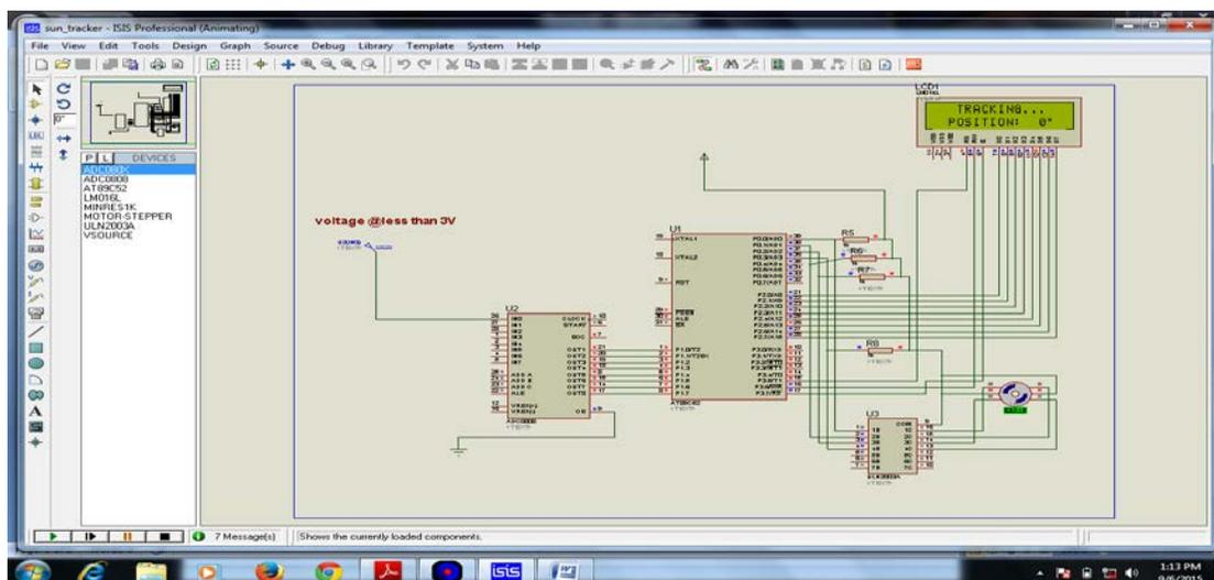
Fig 4.6: LCD showing position of panel at  $V_{in}$  less than 3V.
