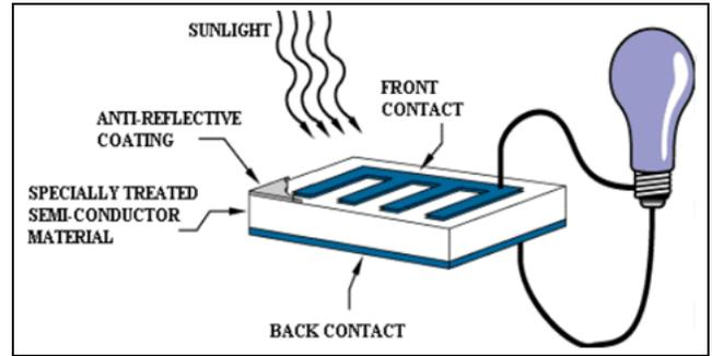
**Fig 2.1:** Basic solar cell operation
