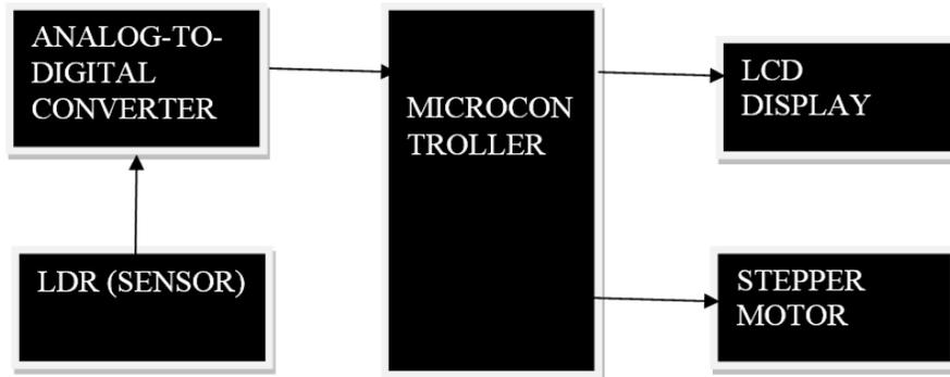
**Fig 3.1:** Block diagram of sun tracker
