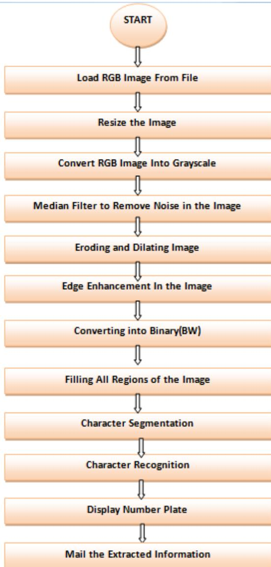
Fig 2: System Block Diagram
