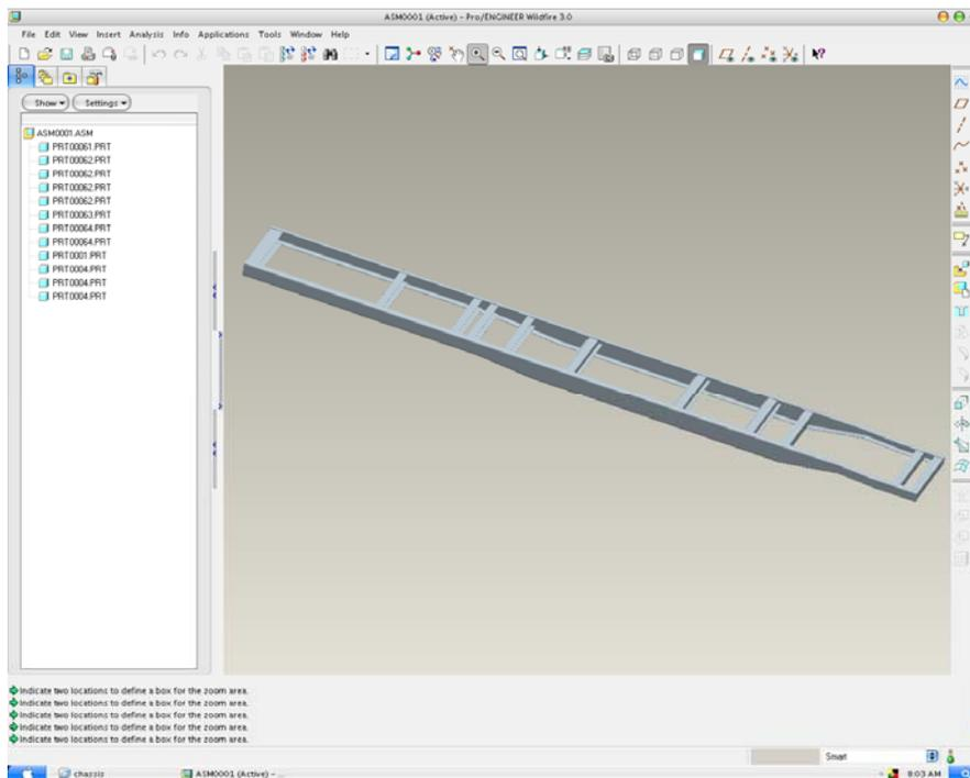
**Fig 1:** Model of chassis assembled in PRO-Engineering
