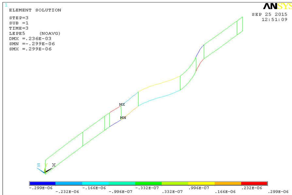
**Fig 2:** Maximum strain developed on chassis
