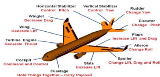
Fig 1: Airplane parts and its function
