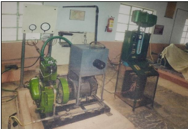
Fig 2: Kirloskar Single Cylinder Diesel Engine
