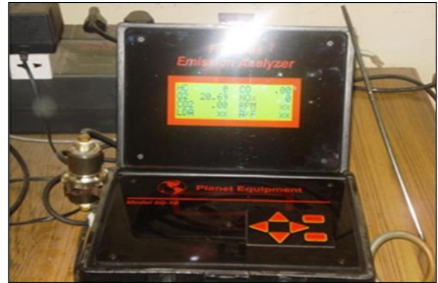
Fig 3: Exhaust Gas Analyzer
