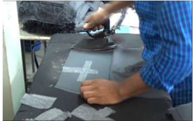
Fig 3: Press fuse to back darts (before)
