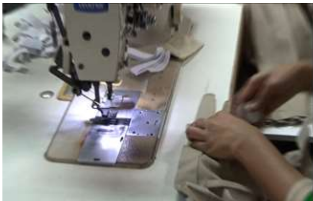
Fig 1: Attaching elastic to tunnel waist band (before)
