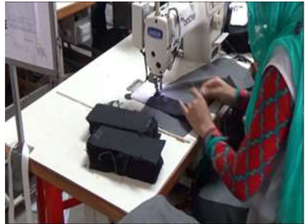
Fig 7: Attaching facing to pocket (before)
