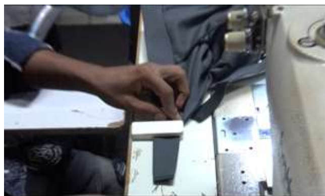
Fig 2: Attaching elastic to tunnel waist band (after)
