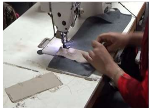
Fig 8: Attaching facing to pocket (after)
