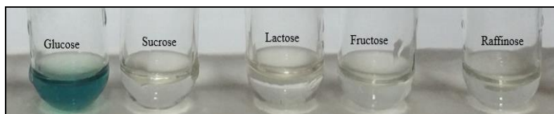
Fig 5: Color changes observed in the glucose determination method with colorimetric method developed by using Fe 3 O 4 MNPs
