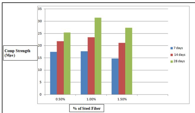
Fig 2: Compressive Strength of Concrete
