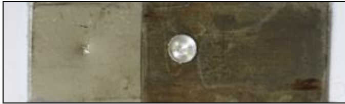
Fig 3: Photograph of a dissimilar AA1050-O/AA6061-T4 lap joint FSSW using 1120 rpm, 7 sec. and 3.05 mm.
