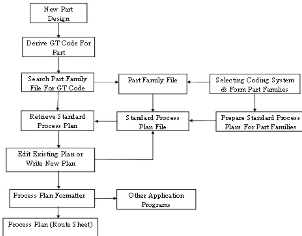
Fig 3: Retrieval/Variant CAPP algorithm. Source: Sehgal (2013)
