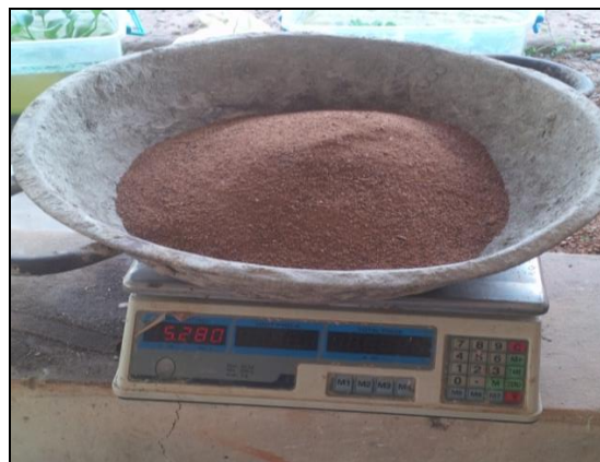
Fig 2: Fine aggregate of 2mm average particle size
