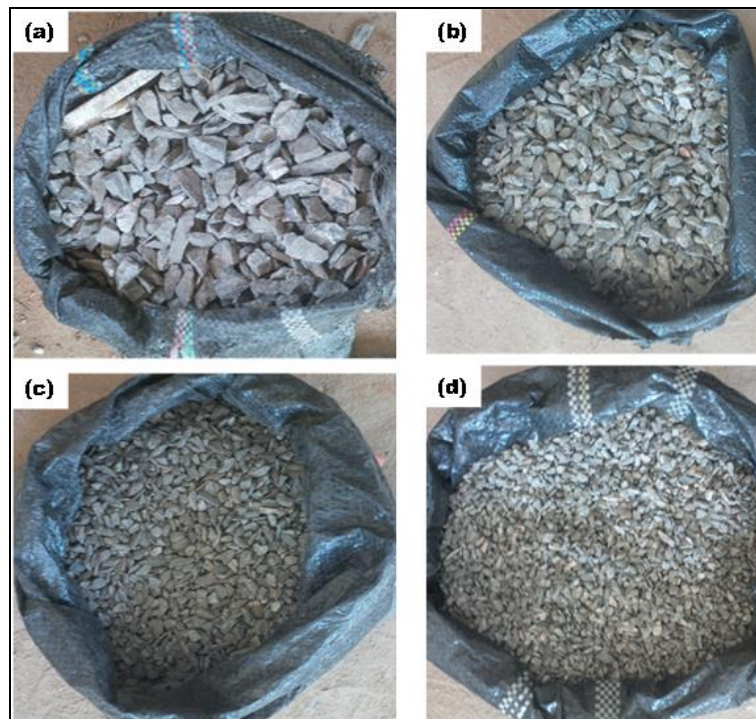
Fig 1: Granite aggregates of different particle sizes (a) 19 mm, (b) 13.2 mm, (c) 9.5 mm, and (d) 6.7 mm
