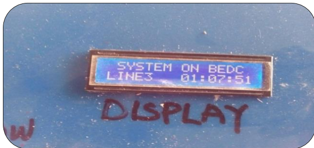
Fig 5: Display during normal operation with public utility available
