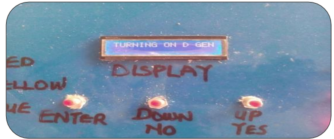
Fig 9: Display during generator turn on
